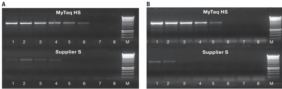
**Fig. 1 Robustness of MyTaq HS in colony PCR**
